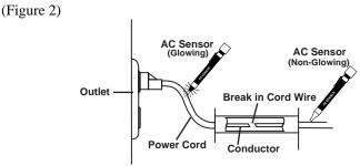
As you move the plastic probe tip away from the electrical source (in this case the wall receptacle), the probe tip will stop glowing at the exact break point in the wire. (Figure 2)
